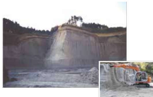
Fig. 1 Shirasu Extraction Process: Shirasu is an eco-friendly building material. Shirasu is already so fine that it does not require a grinding process.
