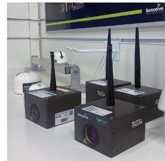
High-precision triaxial tilt sensors
